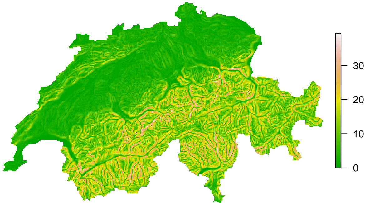
Figure 3: Map of slope in degrees (raster) in Switzerland calculated from elevation map with terrain function.
